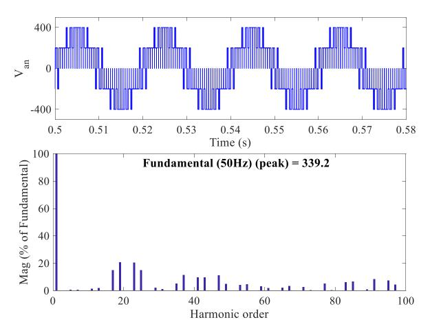
The phase voltage does not contain any triplen harmonic, so the phase current will be absent from it.
