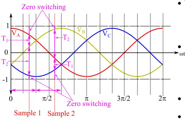
• The space vector PWM is an extension of sine PWM by addition of a common mode voltage.
